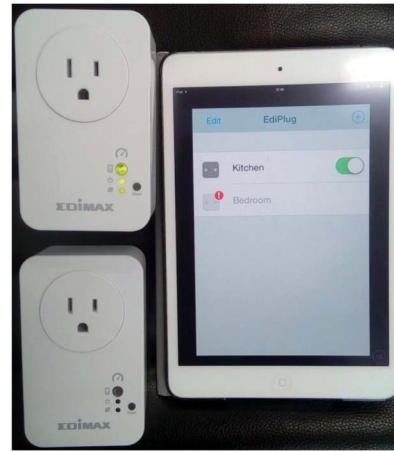
Fig. 1. Edimax plug and iPad installed with the control application.
